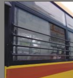
Window Guard Rail
