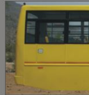
Emergency Exit Door
